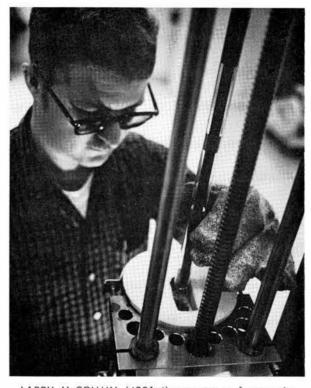
LARRY McCOLLUM (4221-4) operates a furnace in which rolamite glass case material is formed. The system was developed by Ron Snidow and K. D. Boultinghouse of Scientific Glass Lab Section 4221-4.
